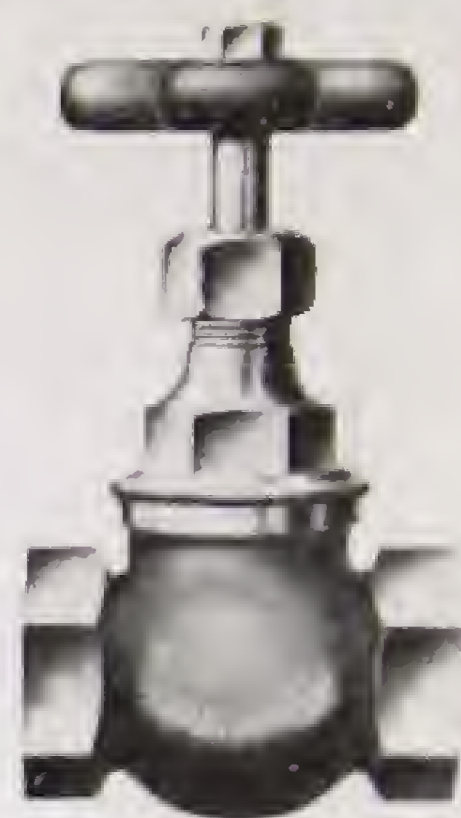
No. B 3154 WHEEL VALVE With renewable composition disc. For steam pressures up to 150 lbs. □". Sizes : ¼ in. to 4 in.
